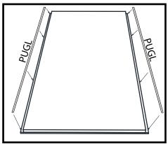
Measure, mark, cut and screw OSB bars onto the wall as shown and accordingly to project requirements. On the back of each panel, apply mounting glue on each side as indicated in gray ("PUGL"). Glue each panel onto the OSB board applying some pressure to it as needed, while protecting front surface finishings. Do the same for the remaining panels.
